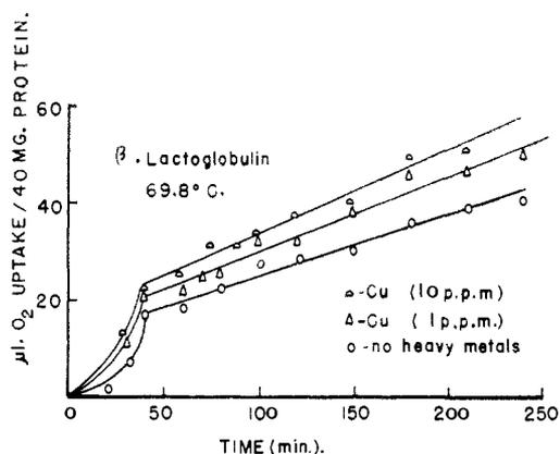
Fig. 3.—Oxygen uptake by  $\beta$ -lactoglobulin during heat treatment. Four ml. of 1% protein sols containing 0.0, 1.0 and 10.0 p.p.m. of copper as copper sulfate was heated in a Warburg apparatus and the total amount of gas taken up was read from the manometers at the indicated times.
