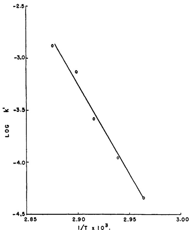
Fig. 7.—Relation between velocity constants and temperature. From the slopes of the line ( $E/2.303 R$ ),  $E$  is calculated to be 80,600 cal./mole.
